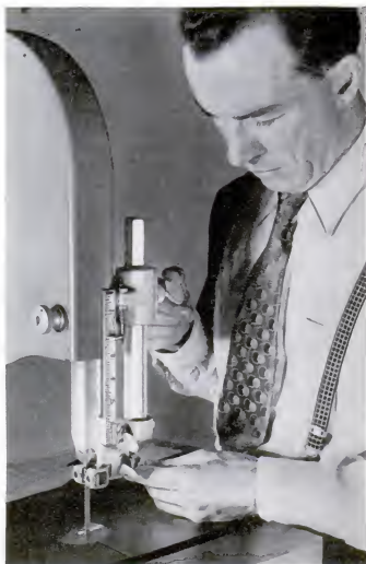
The scale slides with the blade support, and the height is read by means of a pointer on the frame
